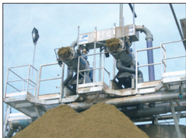
Plant using helicoidal compression for cattle slurries
