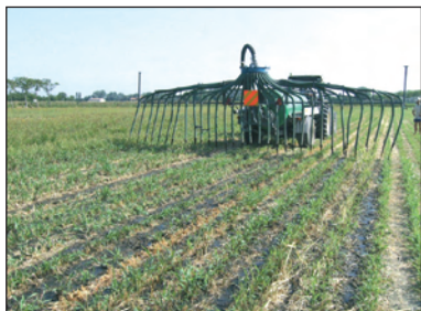
Distribution of covering slurries using low volatile N emission techniques
